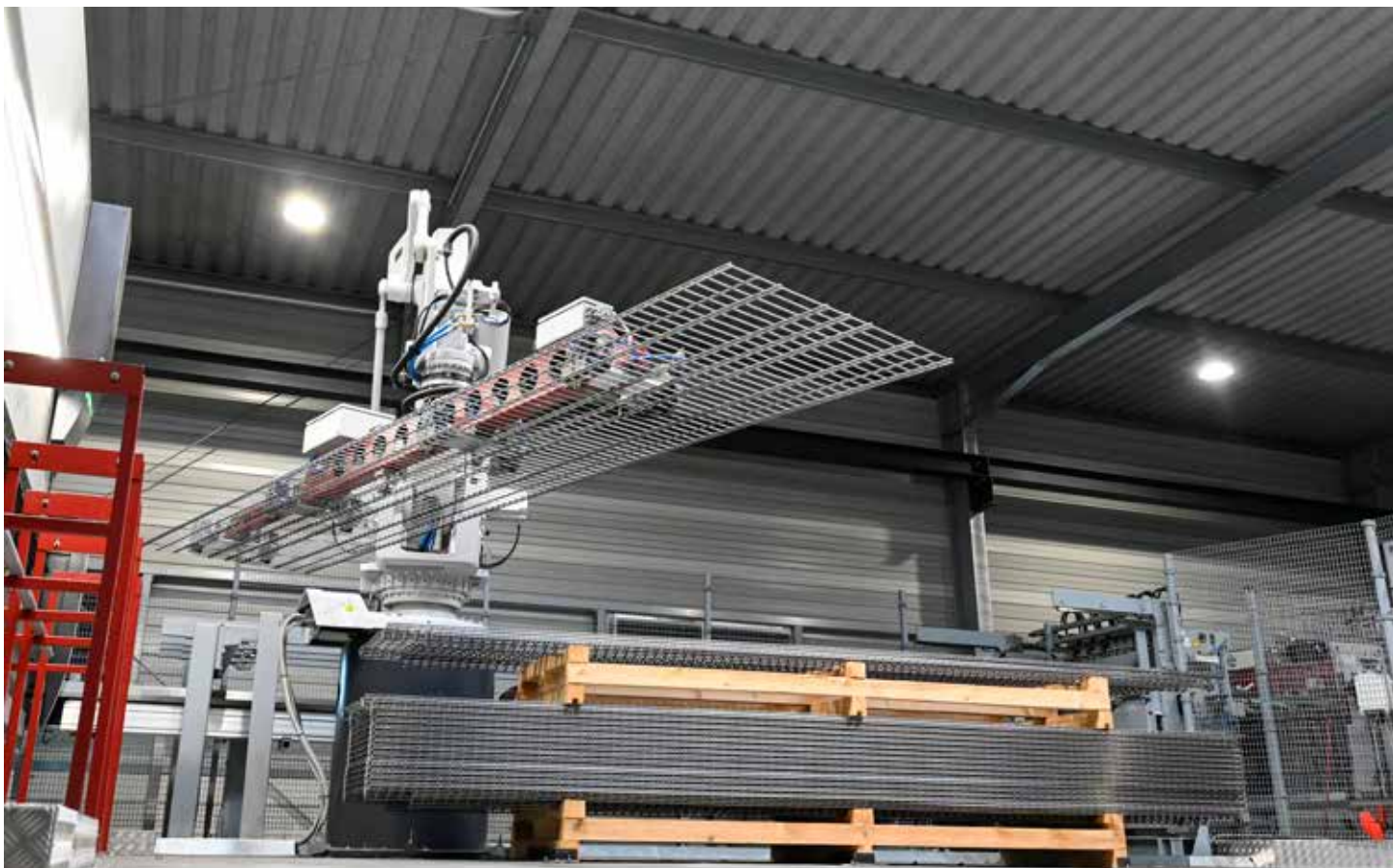
Automated removal of the finished steel mesh mat
